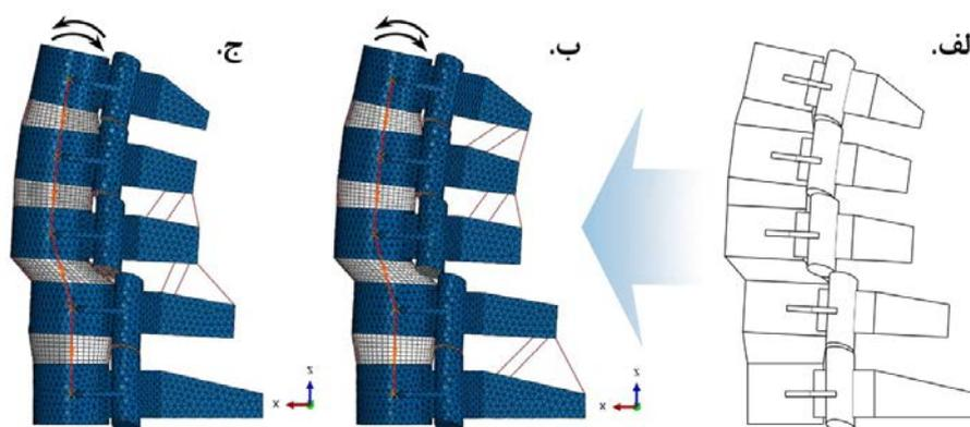
Figure 1. A Model of traumatic injury; A) model designed in CATIA, B) finite element model with ligament tear at the level suffering from a traumatic injury, C) finite element model with ligament tear at the adjacent levels
