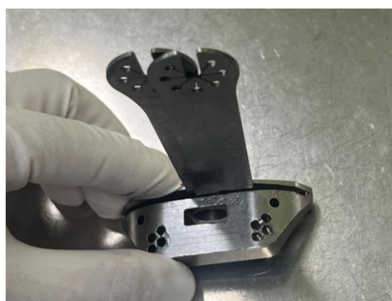
Figure 1: The widths of cutting slot in old set is twice as new one.
