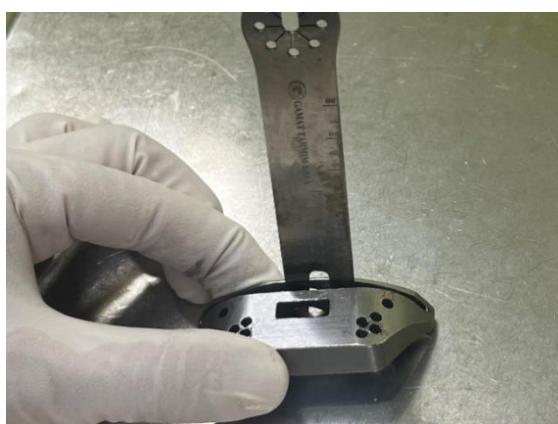
Figure 1: The widths of cutting slot in old set is twice as new one.
